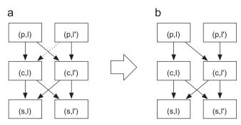
**Fig. 3.** No-contribution elimination. If flow ((p, l'), (c, l)) is guaranteed to have no contributions to generating the values at (c, l), removing the value flow is still safe and precision-preserving.
